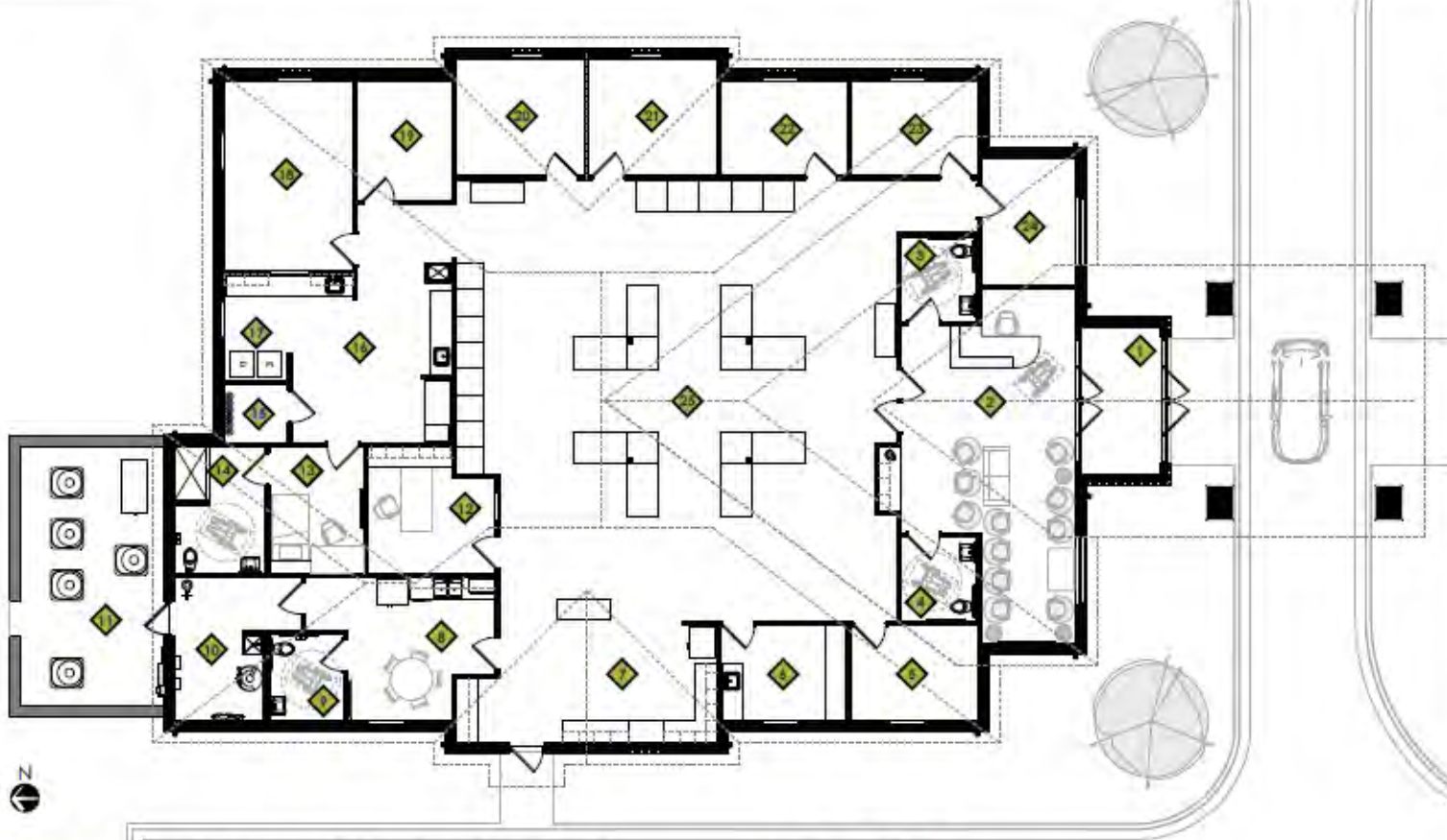
Floor Plan GROSS SQUARE FOOTAGE: 5,409 SF SCALE: 1/16" = 1'-0"
