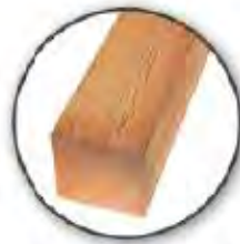
EXPOSED TIMBER FRAMING STAINED & SEALED WESTERN RED CEDAR COLUMNS, BEAMS & TRUSS MEMBERS
