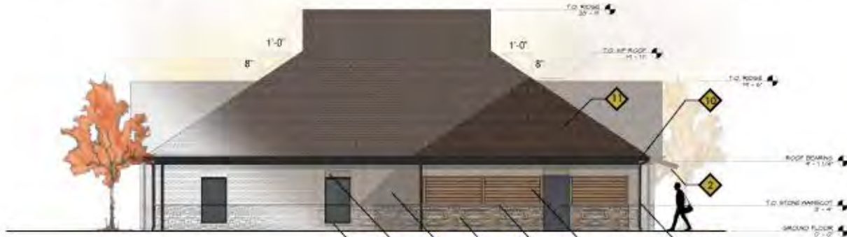
North "Rear" Elevation SCALE: 3/16" = 1'-0"
